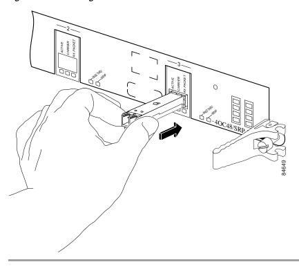
Figure 29 Installing a Slide Tab SFP Module
